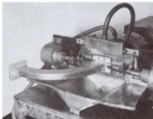
Multi-spindle Drill For True-tolerance Flange Hole Pattern
