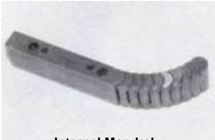
Internal Mandrel Maintains Precise Dimensions During Bending
