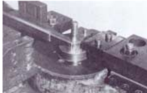
Mandrel In Place On Bending Machine
